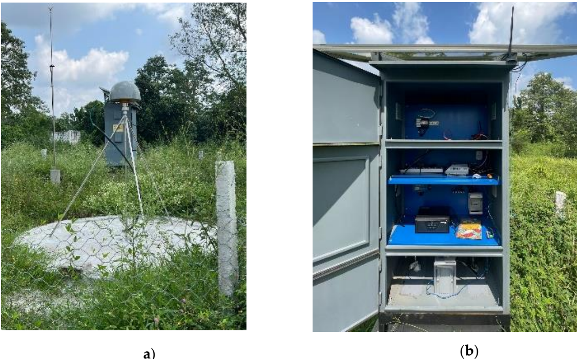
Figure 1: Recently established CORS station (PLWA). (a) CORS Station Monument (b) CORS Station Accessories
