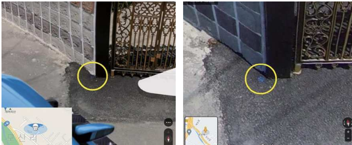
Figure 11 Example showing visibility differences in boundary markers, Road View (left) vs. self-constructed Road-View (right)
