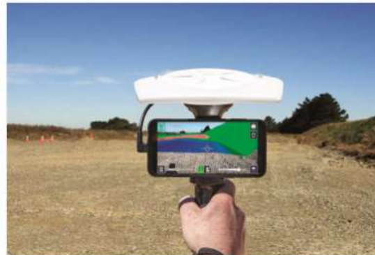
Using augmented reality surveyors can see how a plan is likely to affect the surrounding environment
