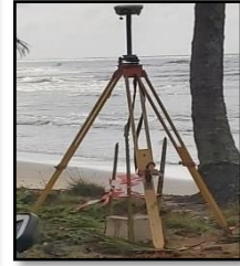
Figure 6: Static GPS mounted on pillar
