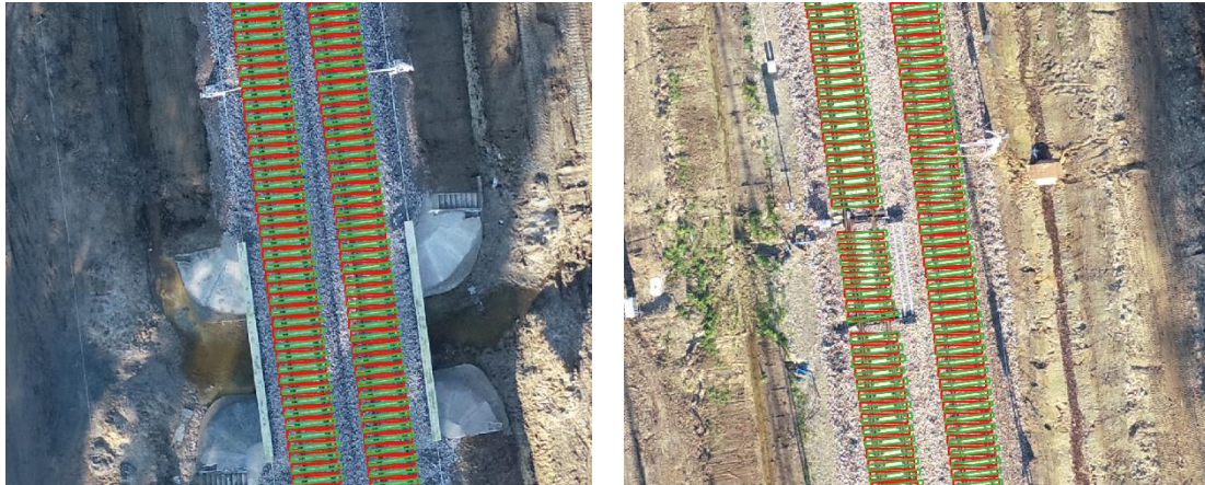
Figure 5 Examples of prediction on a test dataset for the second approach. The green bounding boxes are references; the red boxes are sleeper predictions.
