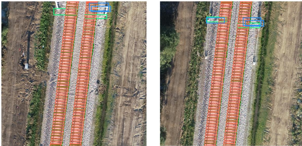
Figure 3 Examples of prediction on a validation dataset. The green bounding boxes are references, the red boxes are sleeper predictions, and the blue bounding boxes are traction pole predictions.
