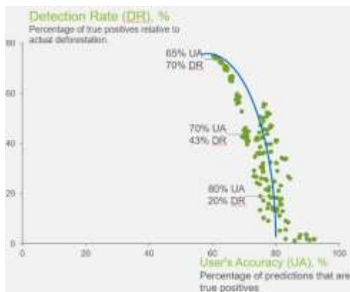
Figure 7: Example relation between user's accuracy and detection rate. Note: this figure merely aims to illustrate the relation and is not portraying the actual model performance.
