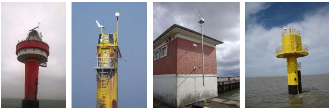
Figure 1: Photos of permanent GNSS antennas at the stations Leuchtturm Alte Weser, Wangerooge-Nord, Wilhelmshaven, Neuer Vorhafen operated by the Waterways and Shipping Office Weser-Jade-Nordsee and the station Knock operated by the Waterways and Shipping Office Ems-Nordsee
