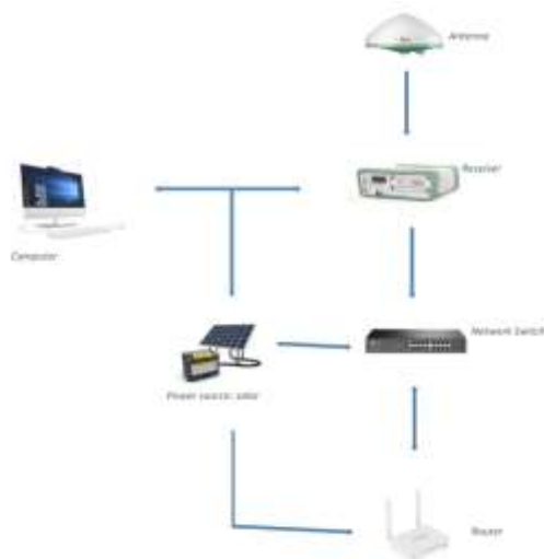
Figure 4: LiSAGNet System Architecture
