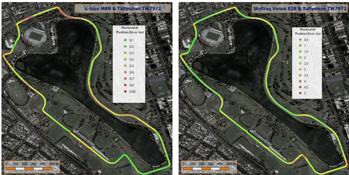
Figure 7. u-blox (left) and SkyTraq (right) Albert Park test with Tallysman TW7972 antenna.
