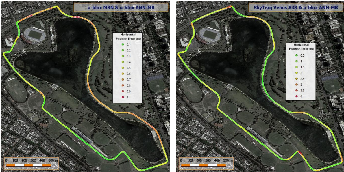
Figure 8. u-blox (left) and SkyTraq (right) Albert Park test with u-blox ANN-MB antenna.
