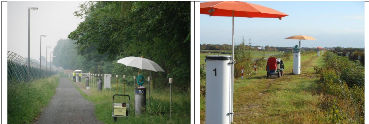
Figure 8. Geodetic baselines of PTB Braunschweig and UniBW Neubiberg.
