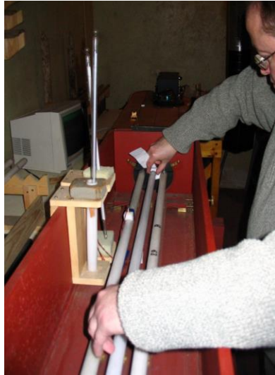
Figure 2. Placing quartz gauges in the comparator box at Tuorla Observatory. Photo: P. Häkli.
