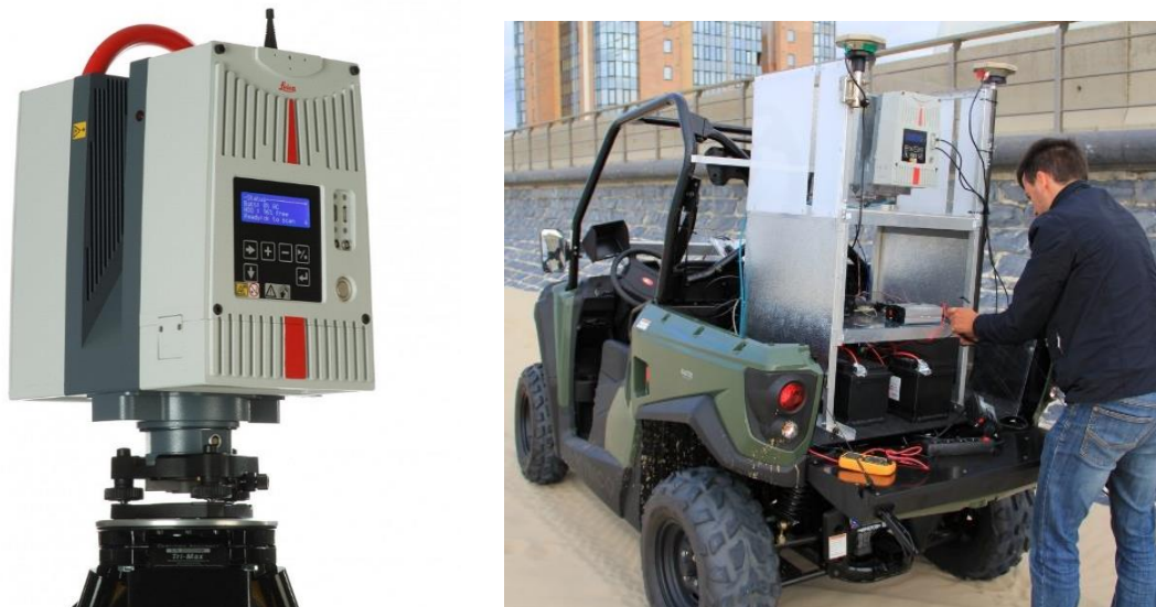
Figure 2.1. Leica (Z&F) HDS 6100 phase scanner (left) mounted on the special service vehicle (right)
