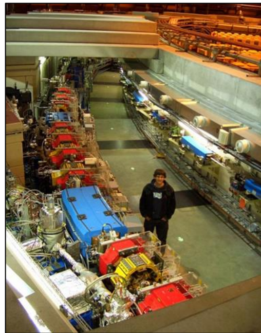
Fig. 1b): Storage ring with colored magnets in the center and photon beam line on the left side.
