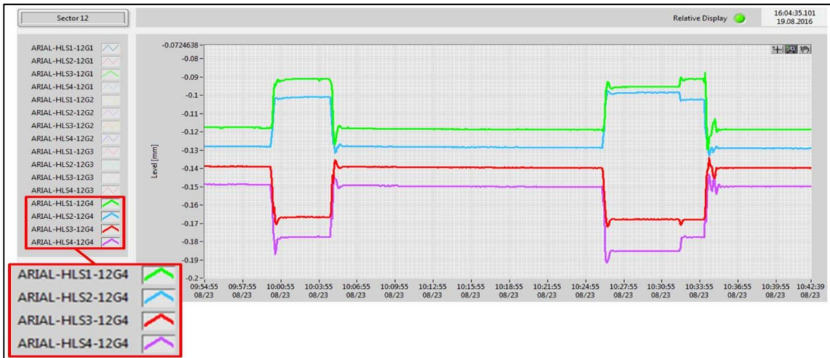
Fig. 6): HLS history data for a girder-displacement test. 2 \times +20 \mu\text{rad} pitch steps were applied according the readout of the motor encoders. Only the HLS sensors of the moved girder are displayed (12G4), showing contrary signal characteristics (2 up, 2 down). The first displacement step is showing the correct signal sequence, whereas the second step suffered from intermittent motor power supply trips at the beginning of the change.
