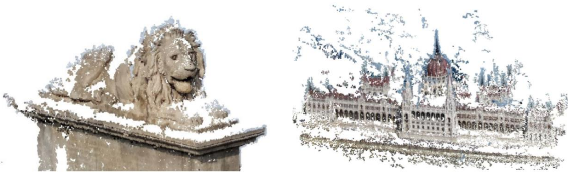
Figure 5: Reconstruction from smart phone images (left), Dense point cloud of the Parliament building after reconstruction from images (right) (source: Somogyi et al., 2016).
