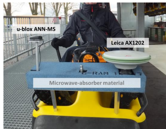
Figure 4: Coaster car with both GNSS antennas fixed on the front part; microwave absorbing foam was used to reduce potential signal reflections from the car's nearby metal parts.
