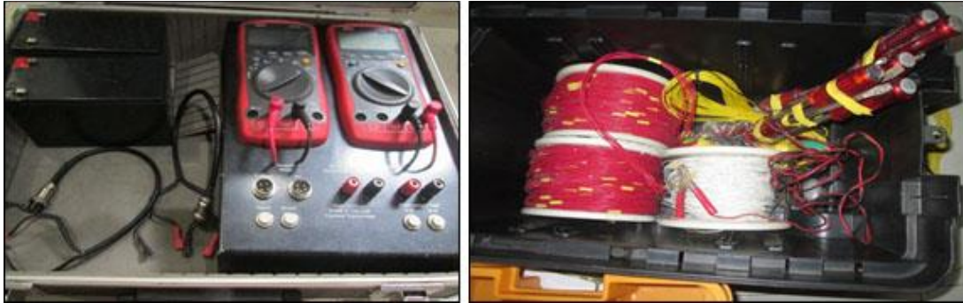
Figure 4. Geoelectricity tools OYO Model McOhm EI 2119C and several additional tools
