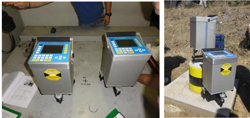
Figure 3. a) Stationing at absolute gravimetric point; b) stationing at points from First Order Gravity Network
