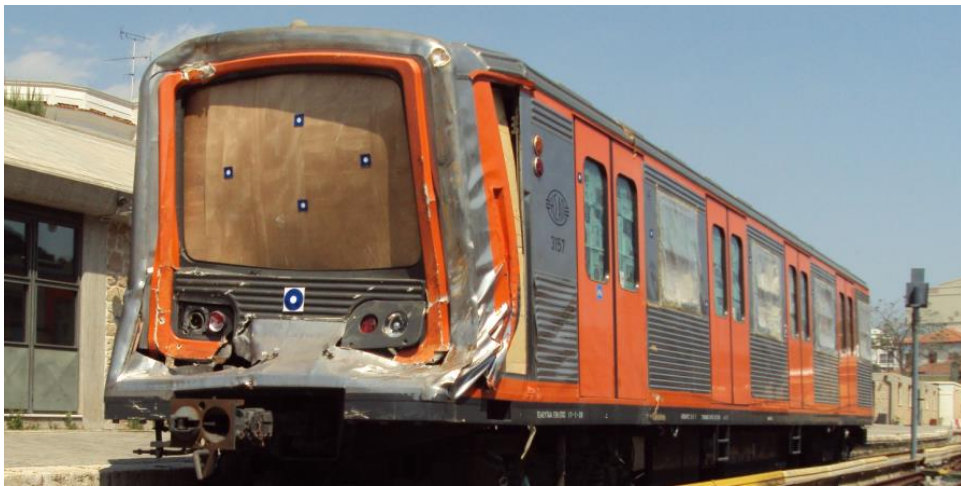
Figure 2. Reflective targets placed on the damaged train carriage
