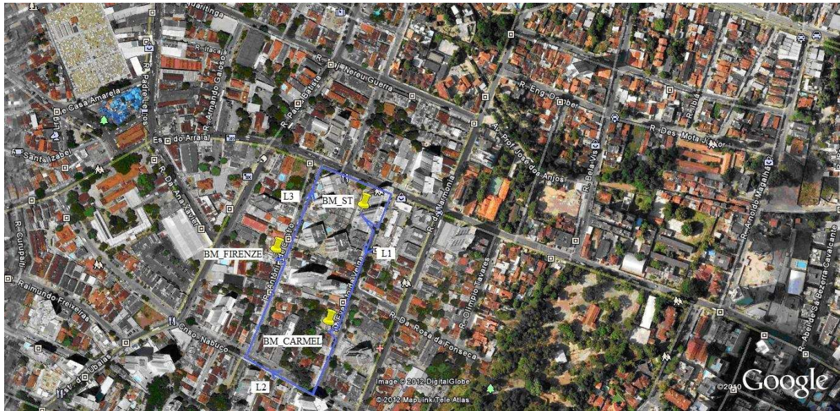
Figure 1: Aerial view of the lines L1, L2 and L3 of the geometric leveling and the field points materialized by BM. Source: Google (2010).
