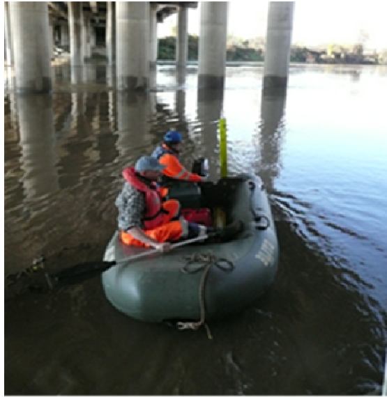
Figs. 6,7 – The typical equipment used in the past by Geo Survey for bathymetry measurements in shallow water. On the right side one can notice the single-beam echo-sound transducer fitted to a graduated pole.
