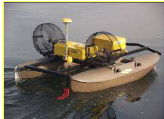
Figs. 1a, 1b – The CatOne family of Unmanned Surface Vessels (USV): rudder-less and air fan propelled.
