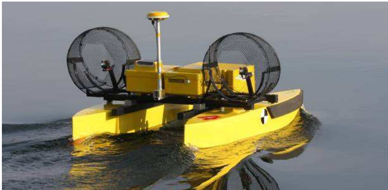
Fig. 9 – The twin-hulls, flat bottom, rudderless configuration of the robot-boat CatOne
