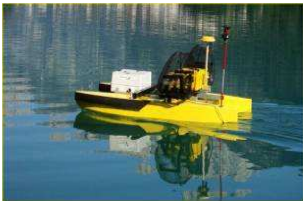
Figs. 1a, 1b – The CatOne family of Unmanned Surface Vessels (USV): rudder-less and air fan propelled.
