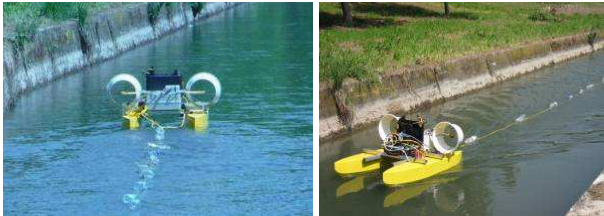
Figs. 14a,14b - The aerRobotix CatOne robot boat tows the electrode array during tests in a canal
