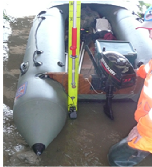
Figs. 6,7 – The typical equipment used in the past by Geo Survey for bathymetry measurements in shallow water. On the right side one can notice the single-beam echo-sound transducer fitted to a graduated pole.
