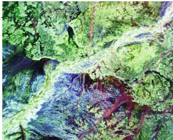
SIR-C color composite image of the Ubar fortress surrounding area: L-HH as red, C-HH as blue and L-HV as green
