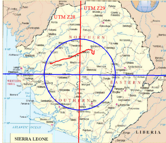
Figure 10. UTM projection and the proposal of stereographic projection for Sierra Leone
