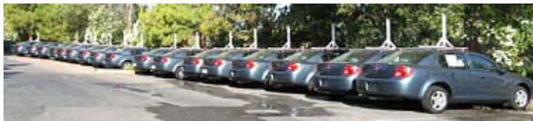
Google Street-View Camera Car Fleet - Each car is equipped with GPS and six stereo cameras taking images at 360° every 2 metres.
