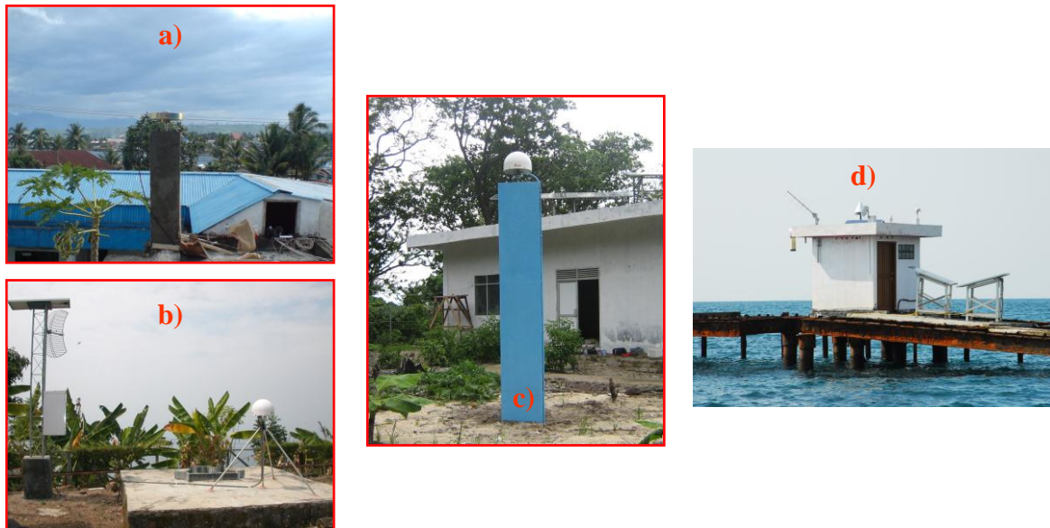
Figure 2. The IPGSN geodetic monument types: a) on the top of concrete roof; b) stainless-steel rod; c) concrete pillar; d) on a tide gauge station.
