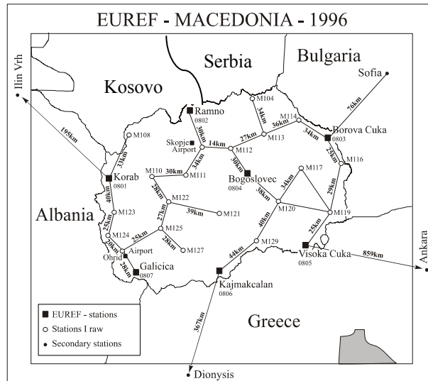
Figure 9. Connecting of Macedonian GPS network with EUREF – year 1996 (Ribarovski R., 2005)
