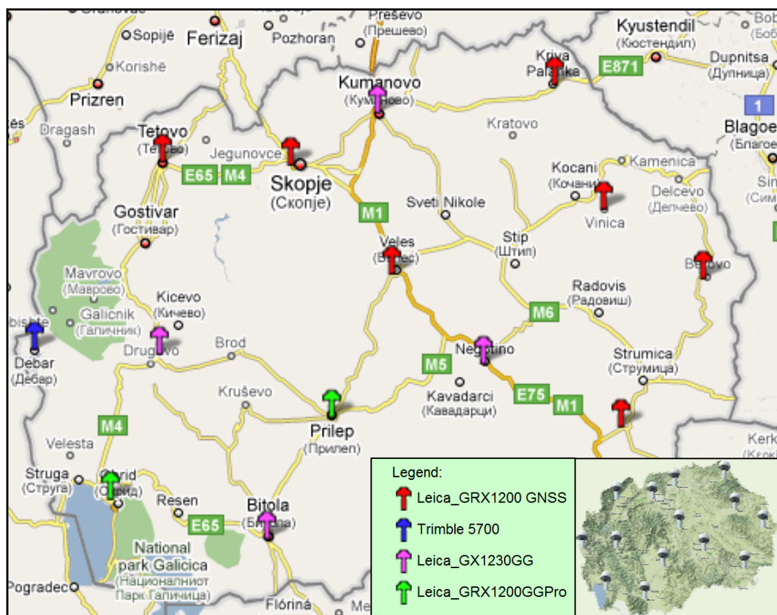
Figure 13. Active GNSS network of Macedonia ( http://makpos.katastar.gov.mk )
