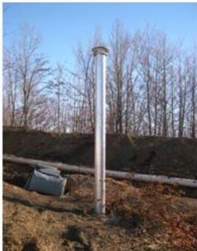
Fig. 5: Example of GPS benchmark – periodic survey
