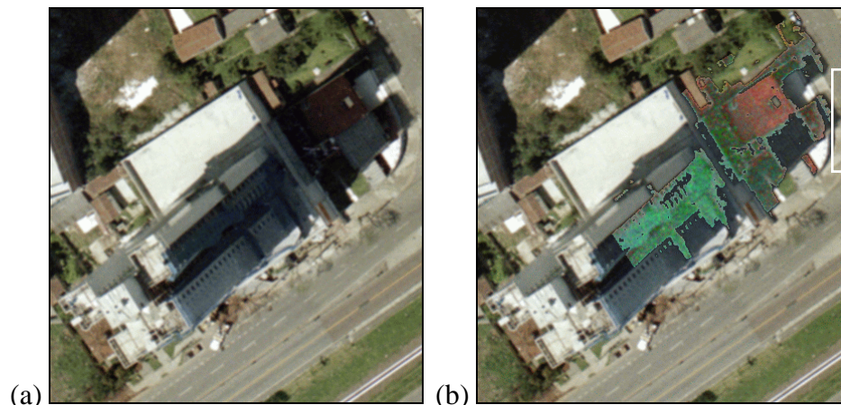
Figure 3-2: (a) Part of the original aerial image showing a shadowed area cast by a building (a); Shadowed area compensated by CAIM (b).
