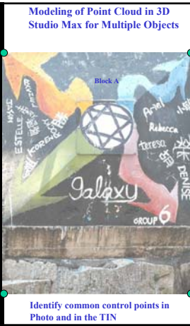
Use control points to fix camera position and then import the photo texture for overlapping
