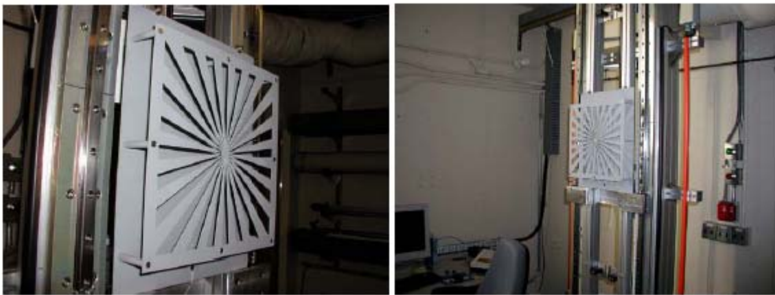
Figure 2. Target for Resolution test
