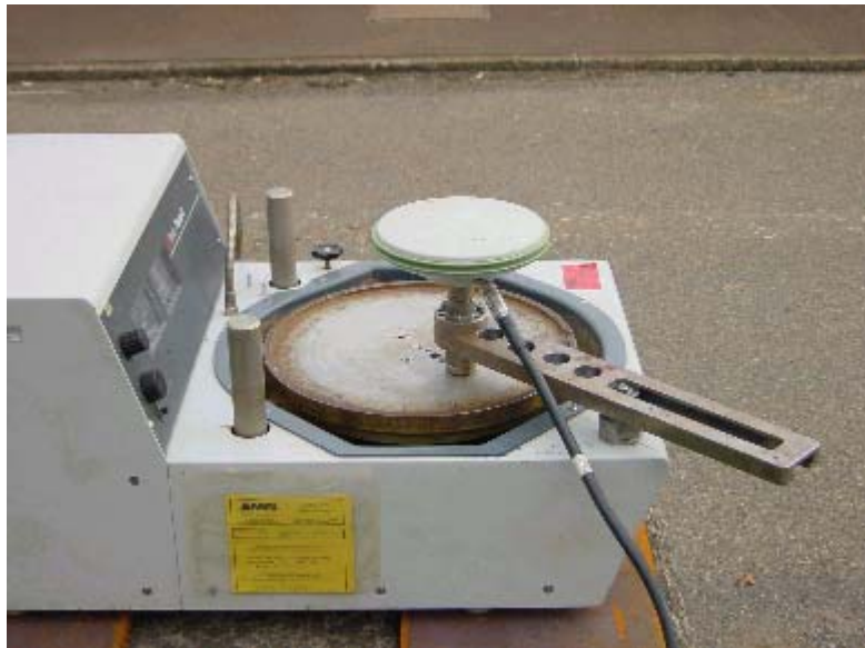
Figure 3 - The turntable with the GPS antenna used in the testing stage
