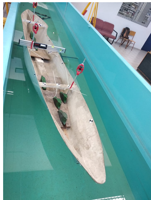
Figure 6. The vessel model in the water tank during the inclining experiment
