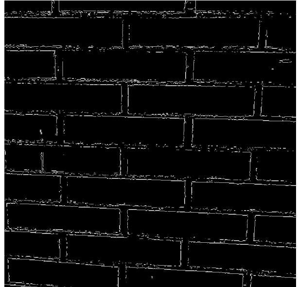
Figure 4. Result of the Sobel filter on a portion of video frame acquired by the drone.
