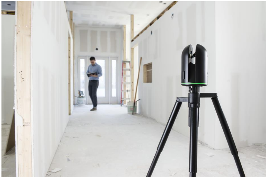
Fig. 4 As-built documentation for renovation
