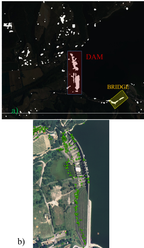
Fig.9.a/b Coherence map and DInSAR measured displacements over the dam classified by average velocity of Corbara dam obtained by COSMO SkyMed images.
