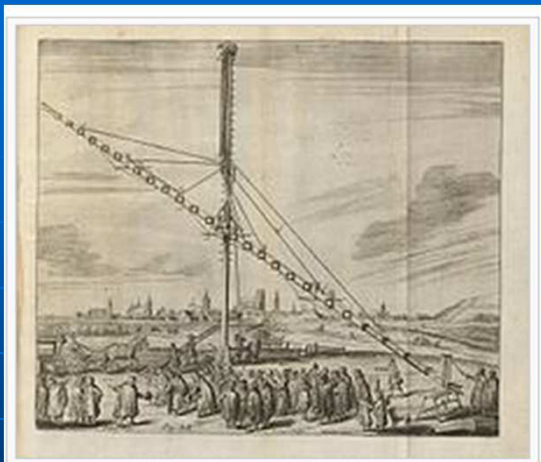
Woodcut illustration of a 46 m (150 ft) focal length Keplerian astronomical refracting telescope built by Johannes Hevelius.
