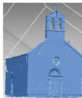
Figure 5 Result of outside laser scanning after data processing (Topić 2005)
