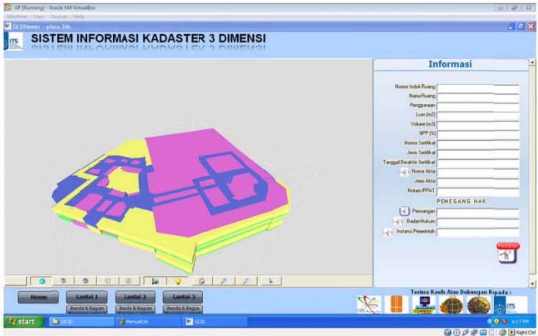
Figure 4. A screen capture of the SIK3D as the LADM implementation prototype
