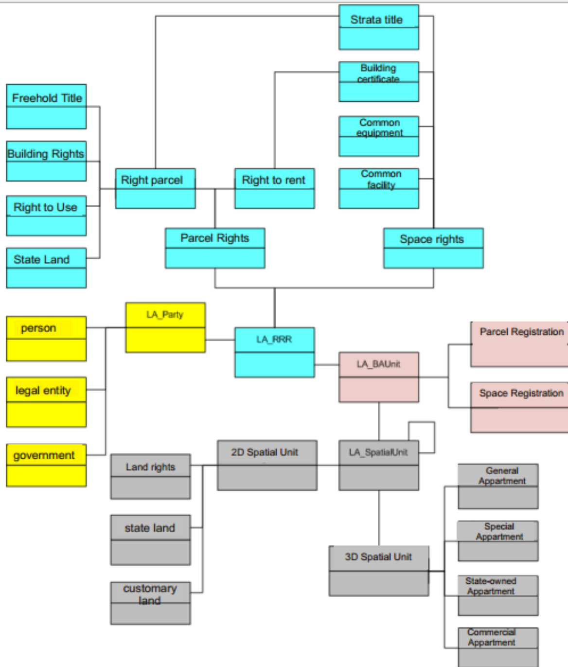
Figure 2. Basic classes of LADM development diagram
