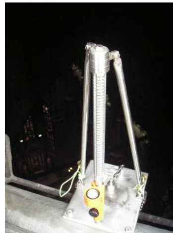
Figure 4. Plate for small leveling rod, optical level or total station.
