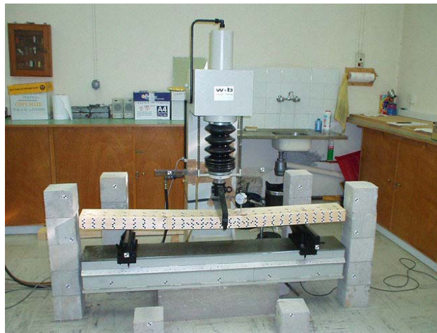
Figure 6: The timber beam under the last loading before the failure
