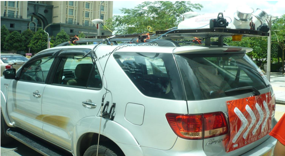
Figure 1: MTLS Dual Laser DynaScan 3 system used
