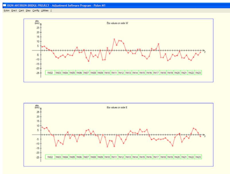
Figure 21: As-built construction error \eta along cantilever
