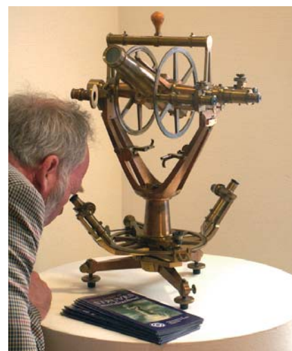
Jan de Graeve with the Reichenbach theodolite used on the Arc measure and recently rediscovered.
